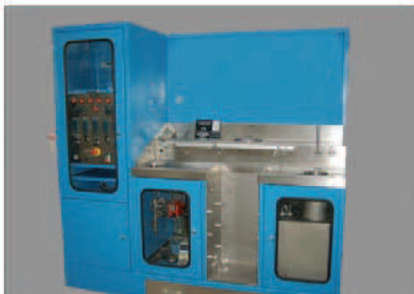
IFTS, Inc.'s Global Fuel Water Separation (FWS) Filter Efficiency Test Stand
